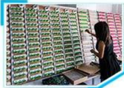
9. Aging test for travel charger
