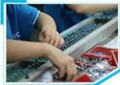
5. Plug in components and parts
