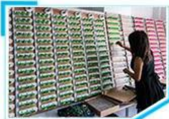
9. Aging test for travel charger
